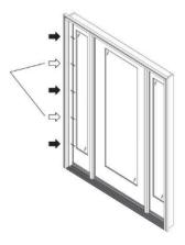
even top to bottom. Finish driving screws tight. Repeat the previous step on the sidelite hinge jamb on the lock mull side of the unit.
