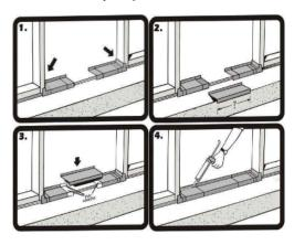
Note: Use only the PVC cement provided in the sill pan kit to glue the pieces together. The sill pan must be sealed to the sub-floor using a high-quality hybrid polymer, elastomeric or polyurethane sealant; Therma-Tru recommends OSI QUAD MAX, but do not apply sealant to the bottom of the sill when using a sill pan.
