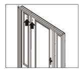
Use a 6 foot level and plumb the hinge side mullion both ways (right to left and inside to outside).
