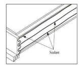
Lay the door unit on edge or face so that the bottom surface of the sill can be caulked. Place very large beads of caulk across the full width of the sill. Additionally, place beads of caulk along the junction of the sill and the jamb and on the bottom surface of the jambs and brickmould.
