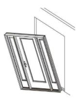
Lift the unit up. With top edge tilted away from opening, center the unit and place sill down onto sill pan or caulk beads and tilt into opening.
