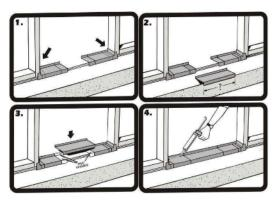
Note: Use only the PVC cement provided in the sill pan kit to glue the pieces together. The sill pan must be sealed to the sub-floor using a high-quality hybrid polymer, elastomeric or polyurethane sealant; Therma-Tru recommends OSI QUAD MAX, but do not apply sealant to the bottom of the sill when using a sill pan.
